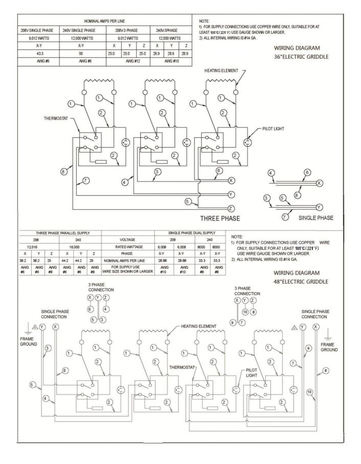
**! WARNING:** This device should be safely and adequately grounded in accordance with local codes, or in the absence of local codes, with the National Electrical code, ANSI/NFPA 70, Latest Edition to protect the user from electrical shock. It requires a grounded system and a dedicated circuit, protected by a fuse or circuit breaker of proper size and rating. Canadian installation must comply with the Canadian Electrical Code, CSA C22.2, as applicable.
